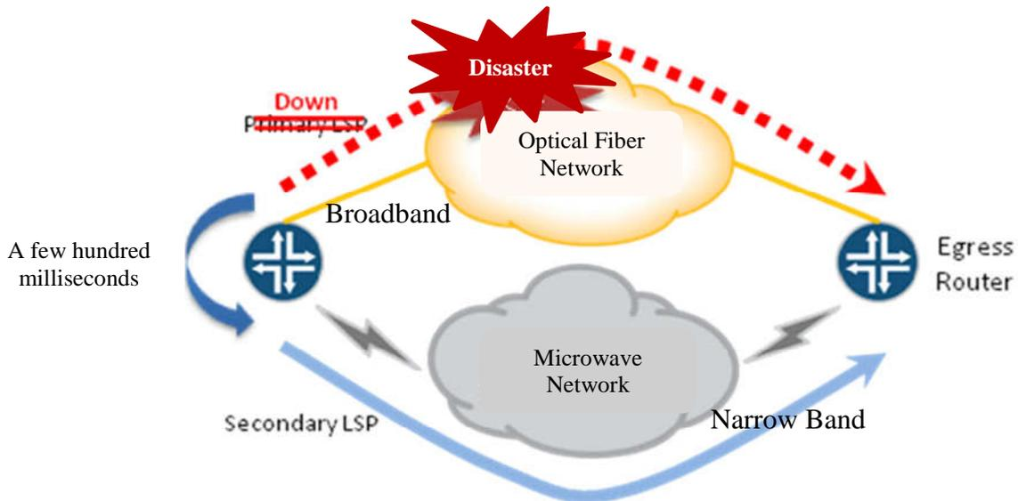
**Figure 5 Route Switching at times of Emergency**
