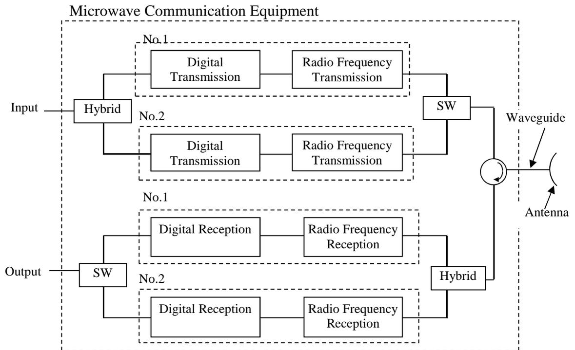
**Figure 3 Example of microwave communication equipment structure**
