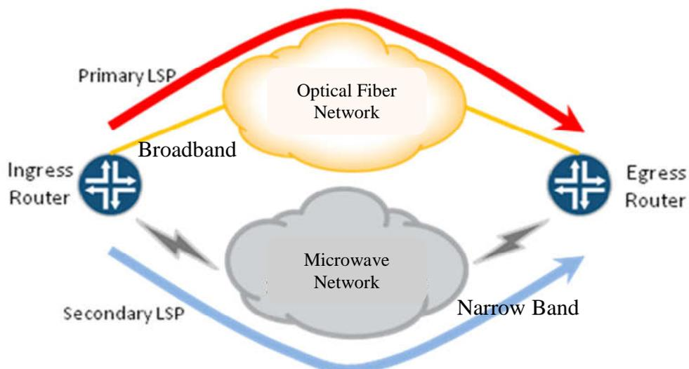
Figure 4 IP Network Structure
